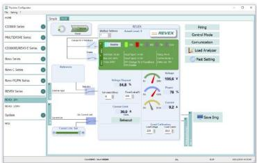
communicates correctly with a power controller, if the connection link is broken the color will become red Address: value used to set the power controller address
