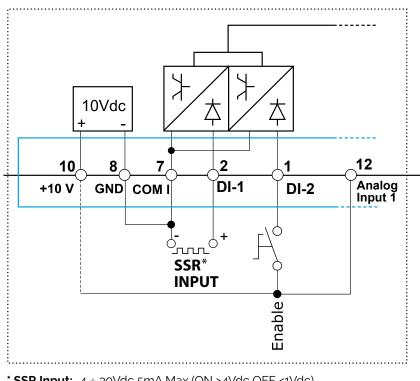
\* SSR Input: 4 ÷ 30Vdc 5mA Max (ON ≥4Vdc OFF <1Vdc) 3HZ Max on time min. 100 ms
