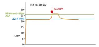
Using the HB Delay parameter, the alarm intervention can be delayed.
