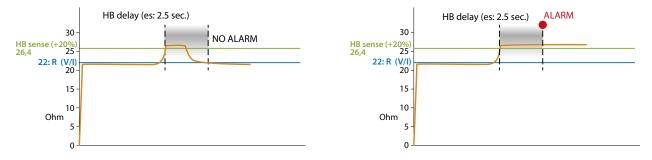
Sensitivity (HB sense) and delay (HB delay) can be varied according to the application (see parameters on pages 32).
