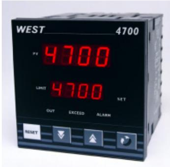
The West 4700 is a safety cut-out, with optional annunciators and alarms. A latched relay cuts process power if safe values are exceeded. A reset is required before continuing.
