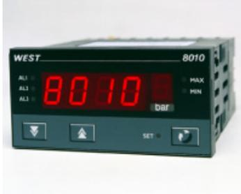
The West 8010 is a 1/8 DIN microprocessor based digital indicator. Available with red or green displays. One latchable relay is fitted as standard, plug-in modules allow two more alarm relays, PV retransmission or transmitter PSU.
