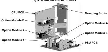
To access modules 1 A or B first detach the PSU and CPU boards from the front by lifting first the upper, and then lower mounting struts. Gently separate the boards. Plug the required option modules into the correct connectors, as shown below.
