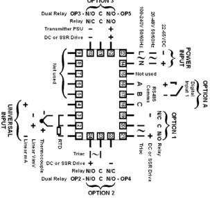
These diagrams show all possible option combinations. The actual connections required depends on the exact model and options fitted.
