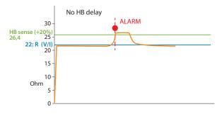
Using the HB Delay parameter, the alarm intervention can be delayed.
