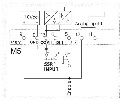
\* SSR Input: 4÷30Vdc 5mA Max (ON ≥4Vdc / OFF <1Vdc) Frequency 3Hz Max - On time min. 100 ms
