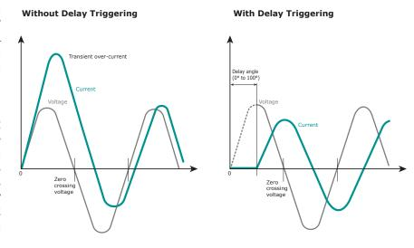
For understand the Delay Triggering firing, we have represented the waves generate by vectors that rotates in counterclockwise:
