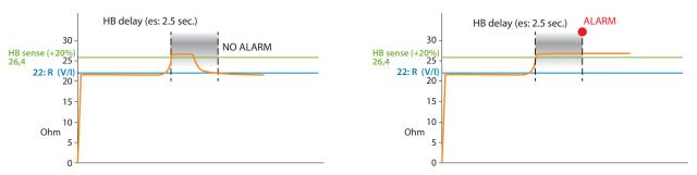
Sensitivity (HB sense) and delay (HB delay) can be varied according to the application (see parameters on pages 43-44).
