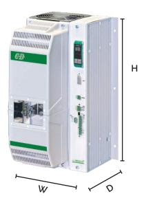
Size: SR21 - 1PH 1400A -1600A-1800A-2100A H: 730 mm, W: 329 mm, D: 347 mm Weight: 34 Kg Standard version with IPO
