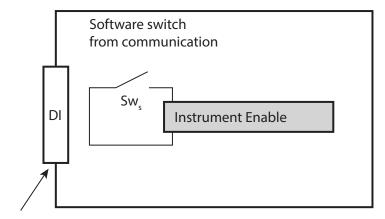
DI Function Configurated like "Not Used" or different from "Enable"
