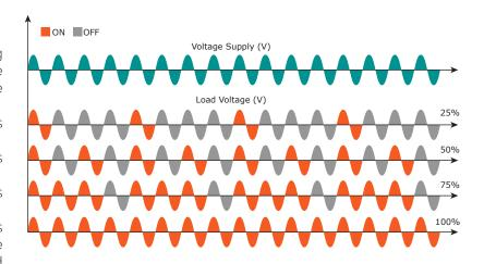
when the sum of rests is one, the unit does one more cycle ON. For this firing is necessary to have analog input. The Single Cycle is used to control the loads with low inertia or for infrared lamps to short wave.
