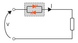
Single phase wiring with inductive load (with REVO C-1PH)
